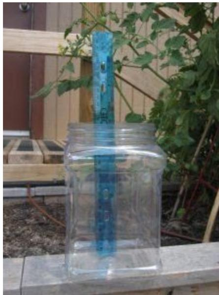
**Rain Gauge:** Since water is vital to plant growth (the rule of thumb is an inch a week for garden plants), growers should be able to keep tabs on rainfall. A rain gauge collects and measures rainfall so that we know how many inches of precipitation we received. The basic components are a collection vessel and a measurer of some type.
